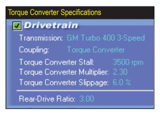
When any torque converter is selected, the *Stall Rpm*, *Torque Multiplier*, and *Slip* percentage fields become active in the DRIVETRAIN category. Use FastLapSim5 built-in selections or DirectClick™ any data field and enter custom values.
